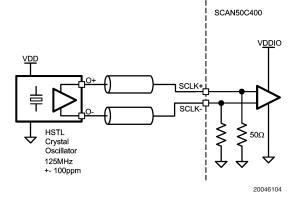
FIGURE 1. SCLK± Driven by HSTL Clock Driver / Crystals
