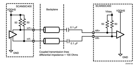
FIGURE 5. High-Speed IO, AC Coupled
